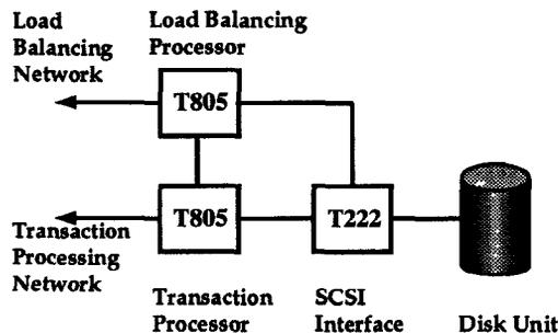
Figure 1, Schematic Diagram of MEDUSA Processing Node
