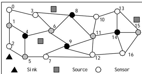
Figure 1 Level-Based Hierarchical Routing Protocol
