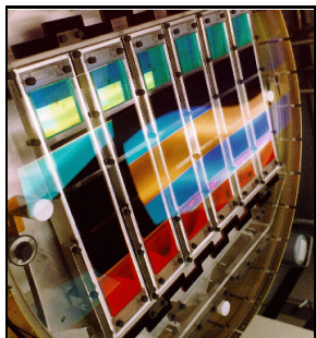
Figure 1: The SDSS photometric camera with the 5x6 CCD array contains 120 million pixels. The CCDs in each row have a different filter attached. As the earth rotates, images migrate across the CCD array. The array shifts in synchrony with this movement, giving a 55 second exposure for each object in 5 spectral bands.
