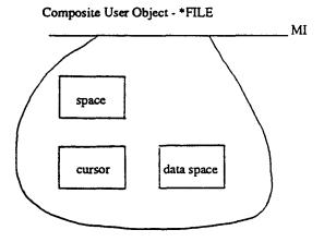
A single membered, non-keyed user physical file consisting of three MI objects, one of type space, one of type cursor and one of type data space.
