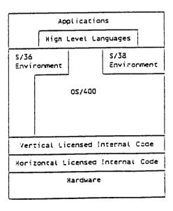
Figure 1. AS/400 Layered Architecture.
