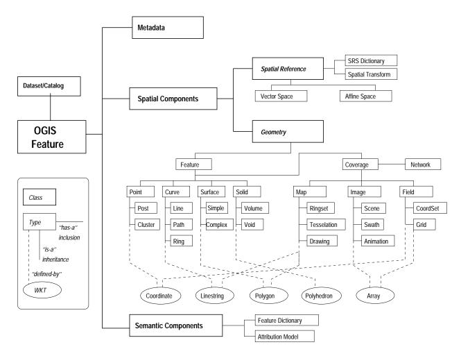
Figure 2. Open GIS Geodata Model class hierarchy.
