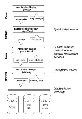
Figure 3. Components of the open environmental information system. **process**.
