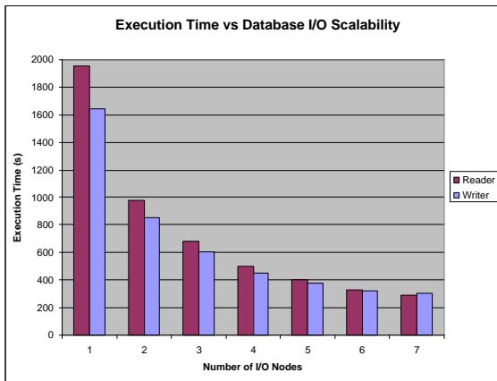
Figure 1. Data I/O Scalability Experiments. “Reader” and “Writer” bars denote the experiments, in which the number of MakoReader and MakoWriter filters is varied, respectively.
