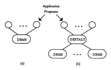
Figure 1: Structure of (a) conventional systems and (b) GESTALT.
