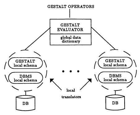
Figure 4: GESTALT system structure.
